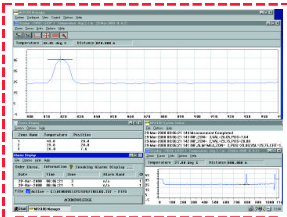
Figure 3 Illustrates the temperature profile display for the entire fibre length and also a numerical display for individual zonal temperatures.
